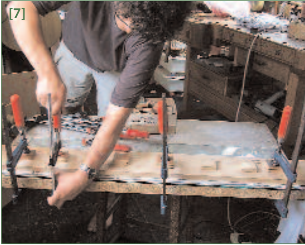
[7] The layers are clamped together to ensure even drying
