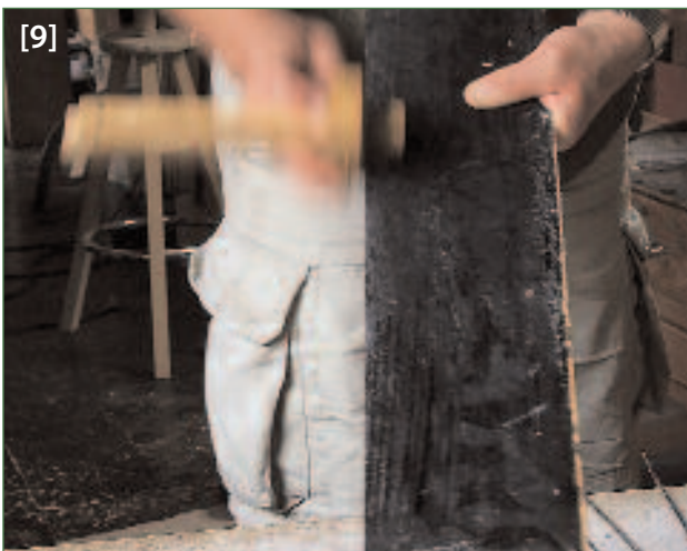
Scoring the sandwich with a marking gauge before cutting
