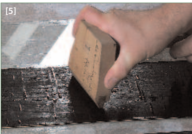
Pushing out the excess glue with a veneer hammer
