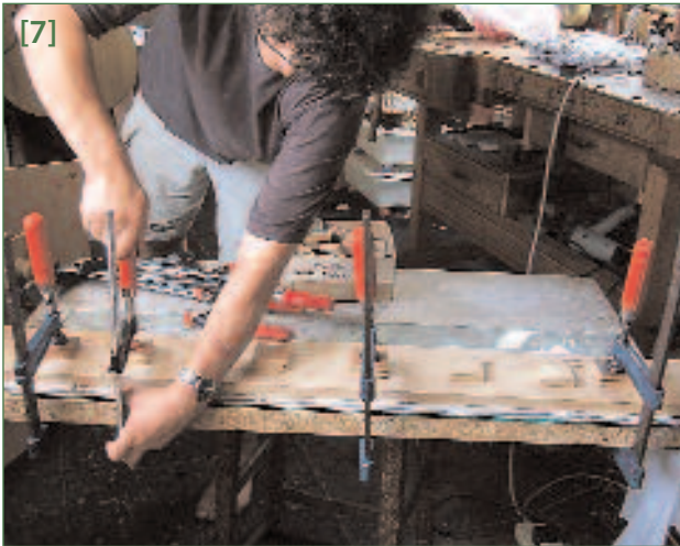
The layers are clamped together to ensure even drying
