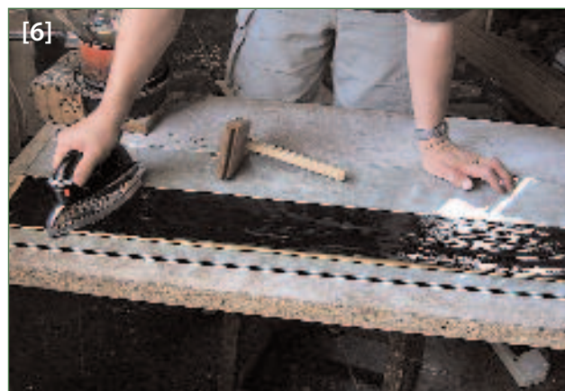
The assemblage is warmed with an iron before excess glue is squeezed out
