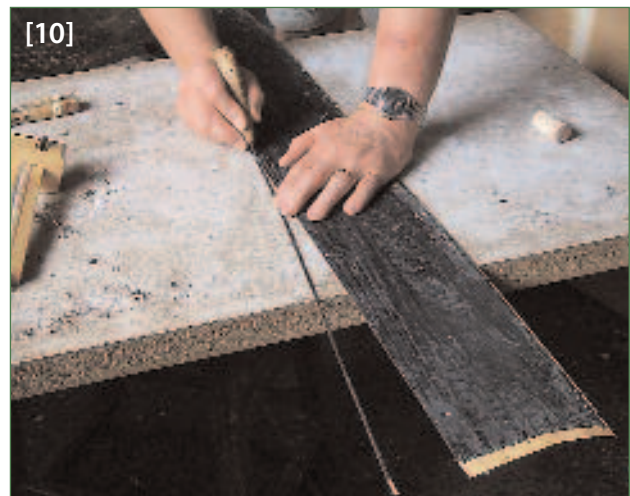
The sandwich is cut into strips while it is still fresh and not too brittle
