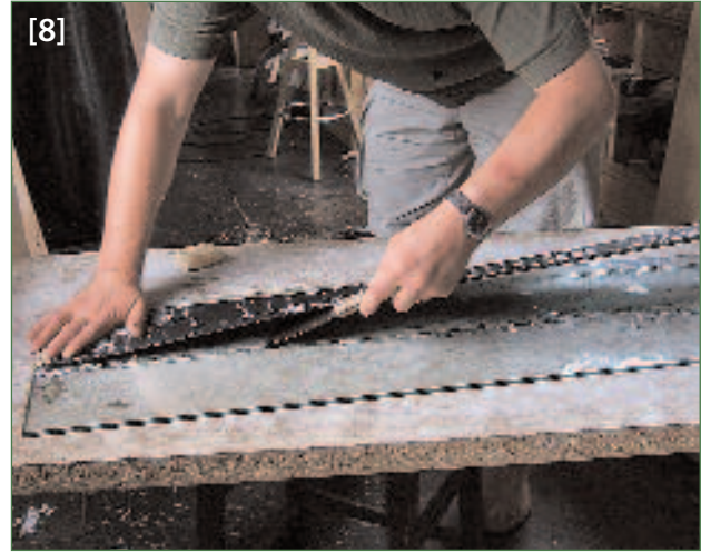
[8] Peeling the sandwich off the glass with a spatula
