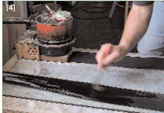
Brushing the first layer of black generously with hide glue
