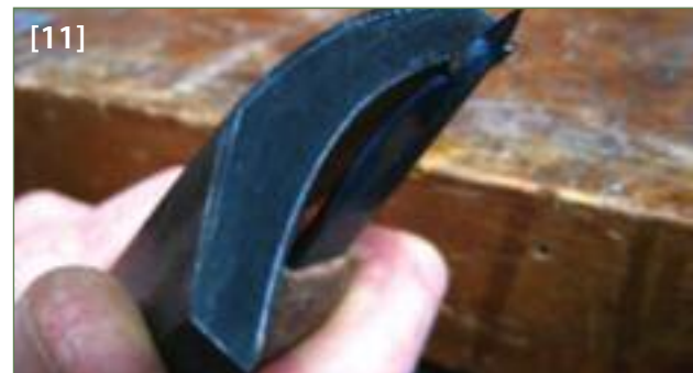
[11] Trimming the underside of the radius with a sharp knife
