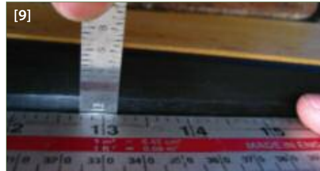
[9] Checking hollowing for string clearance
