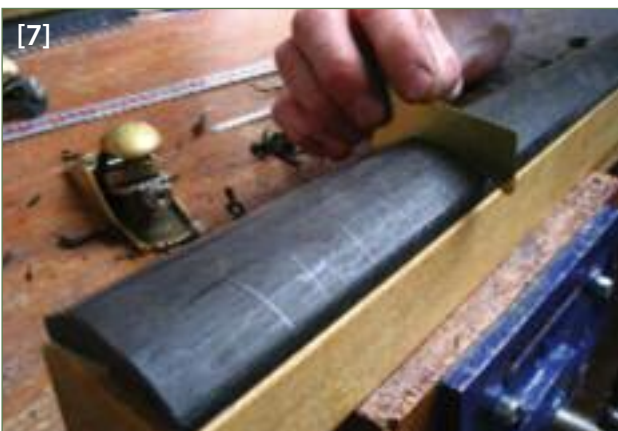
[7] Using a template to check the profile of the radius on the playing surface
