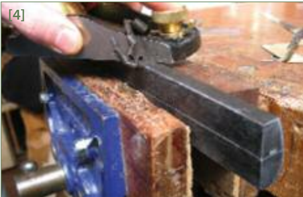
[4] Planing the side so that the fingerboard is square
