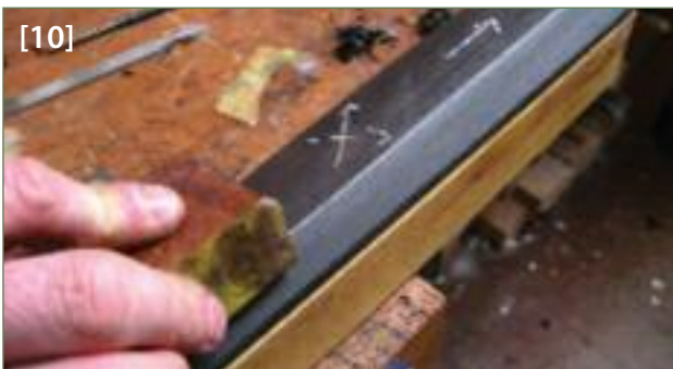
[10] Smoothing the radius of the playing surface with a curved sanding block
