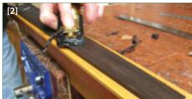
Planing the underside
