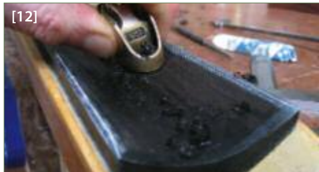
[12] Shaping the underside scoop
