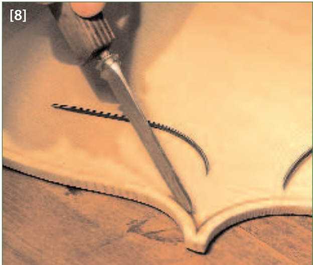
[8] Applying adhesive in the purfling channel with a gluing knife
