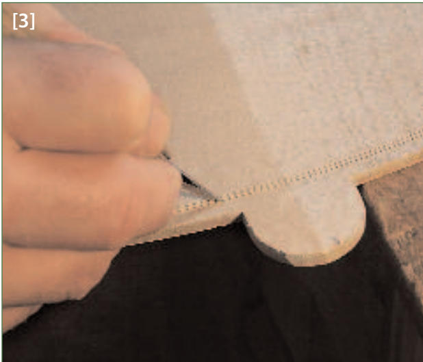
[3] Marking the purfling channel in the button area on the back
