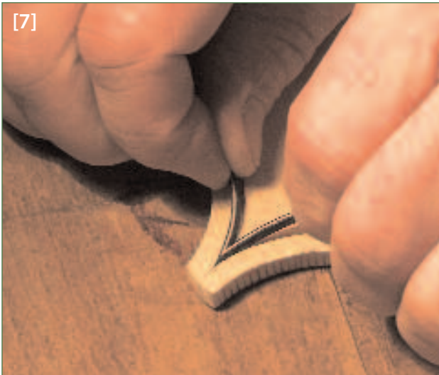
[7] Adjusting the purfling to ensure it fits properly in the corners
