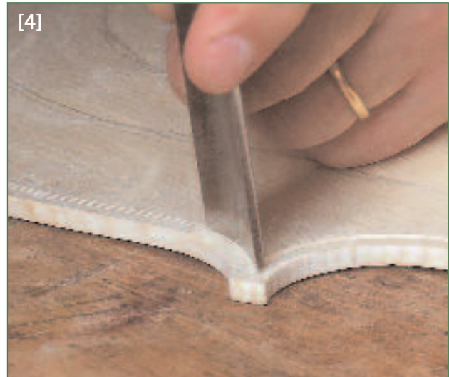
[4] Marking the purfling 'bee-sting' using a wide, shallow gouge
