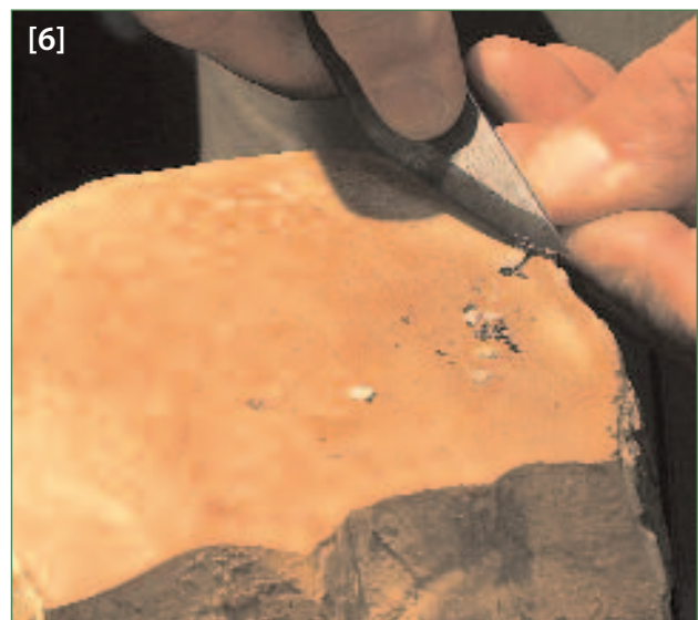
[6] Cutting the purfling strip in preparation for inlaying
