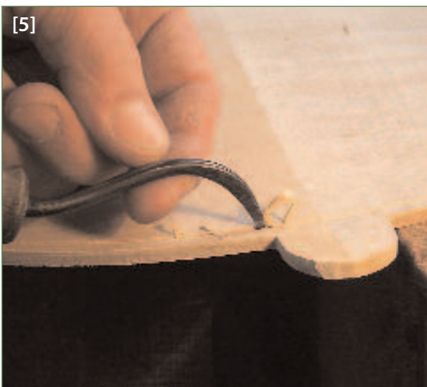
[5] Lifting out the channel to the correct depth with the purfling pick
