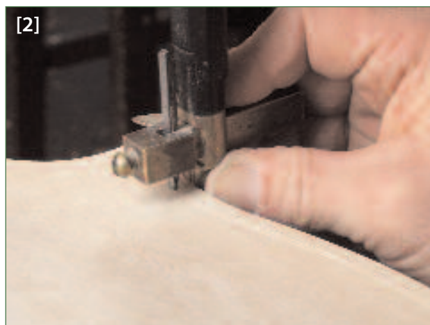
[2] Marking the purfling channel, using the purfling marker to follow the edge
