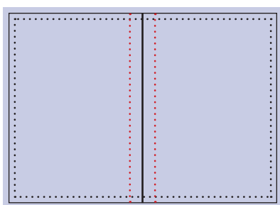
DOUBLE PAGE SPREAD Trim 295mm (h) x 430mm (w) Bleed 301mm x 436mm Type area 260mm x 394mm Gutter 50mm (25mm on each page)
