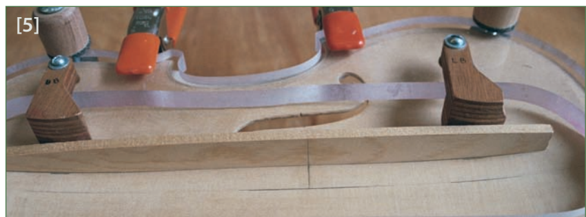
The bass-bar is held in its position at four degrees to the vertical by the guide arms, which are locked with the mounting screws
