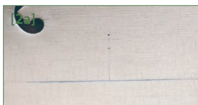
Marking up the inside of the back to fix the position of the bass-bar
