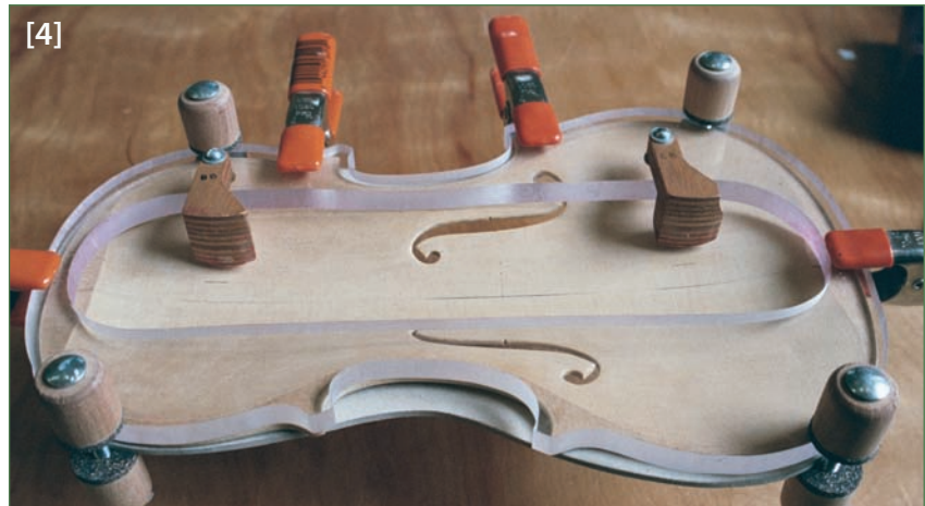
The violin top is held flat against a perspex plate
