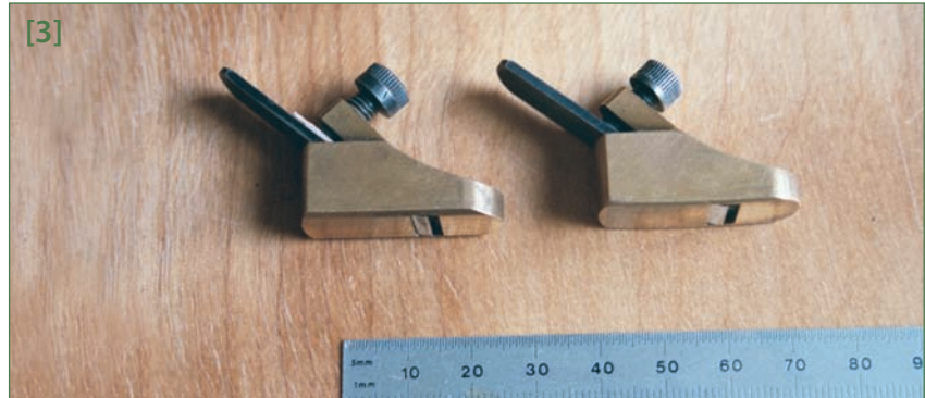
The bass-bar is shaped to fit using thumb planes. The one on the right has a curved sole
