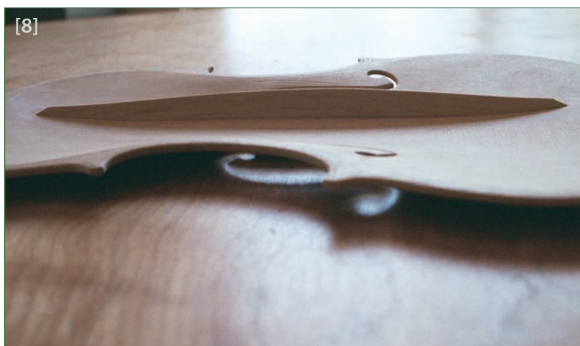
The bar is planed to the desired profile – about 14.5mm in the middle and 3.5mm at the ends
