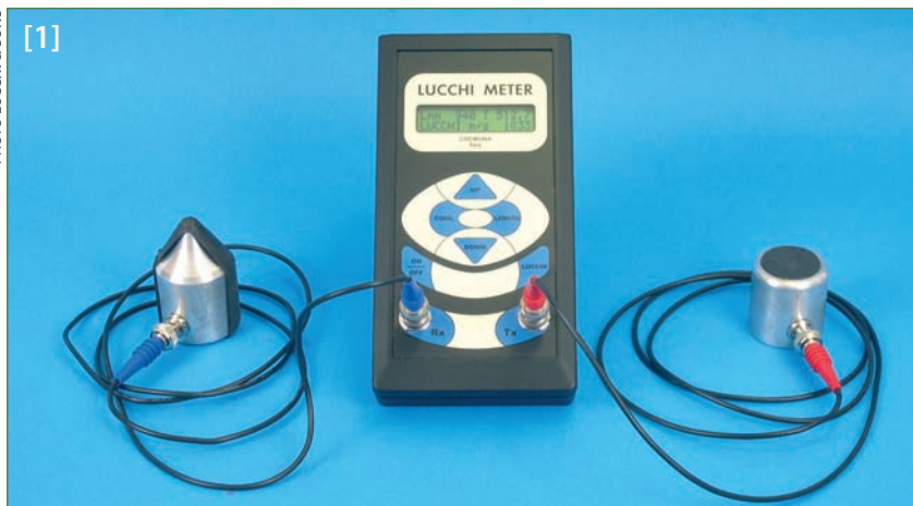
The Lucchi meter is used to measure the speed of sound in wood
