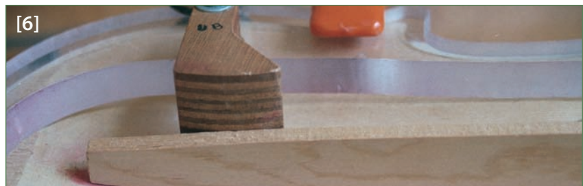
The bar is sprung by about 1.5mm
