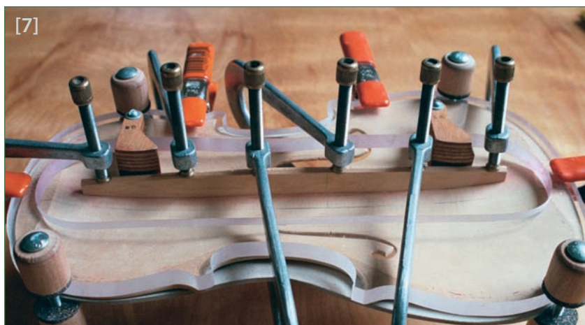
The top of the bar is bevelled so that the clamping force acts in the correct direction
