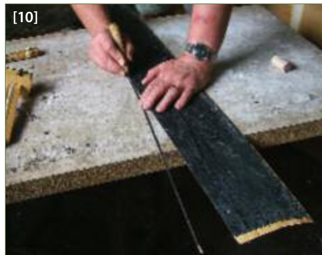
[10] The sandwich is cut into strips while it is still fresh and not too brittle
