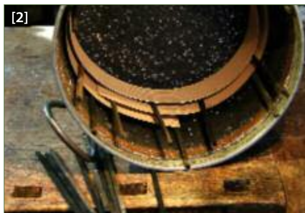
[2] The veneers, separated by distancers, are curled in a large saucepan for dyeing
