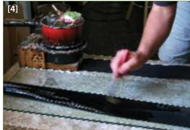
[4] Brushing the first layer of black generously with hide glue
