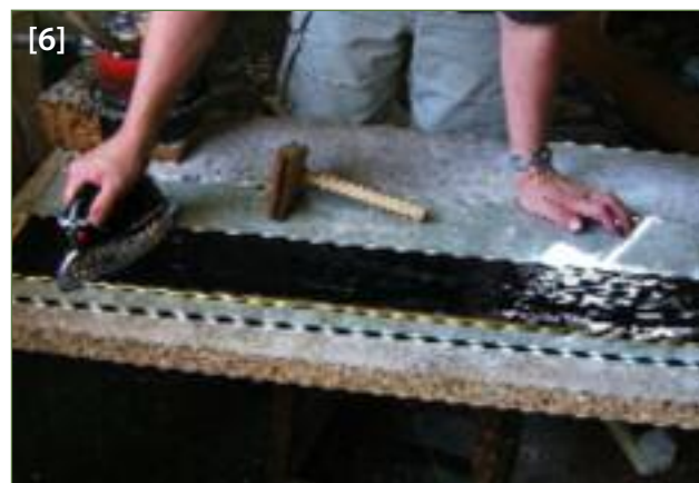
[6] The assemblage is warmed with an iron before excess glue is squeezed out
