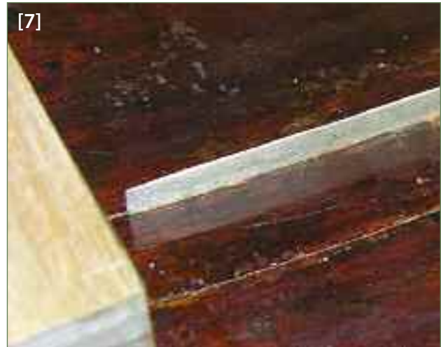
[7] The splint inserted into the crack prior to steaming
