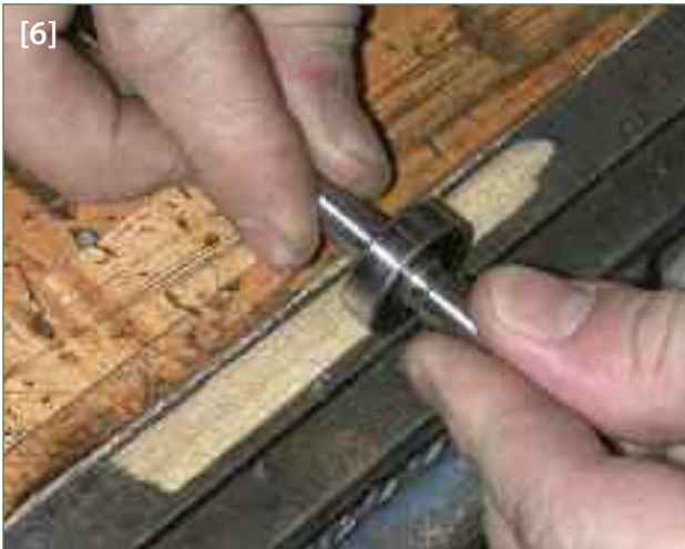
[6] Using a roller to compress the splint against a hard surface
