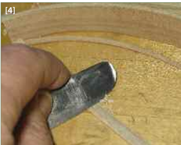
[4] Scraping the splint to thickness
