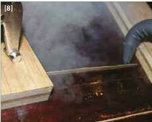
[8] Steaming on each side swells the splint and reactivates the glue
