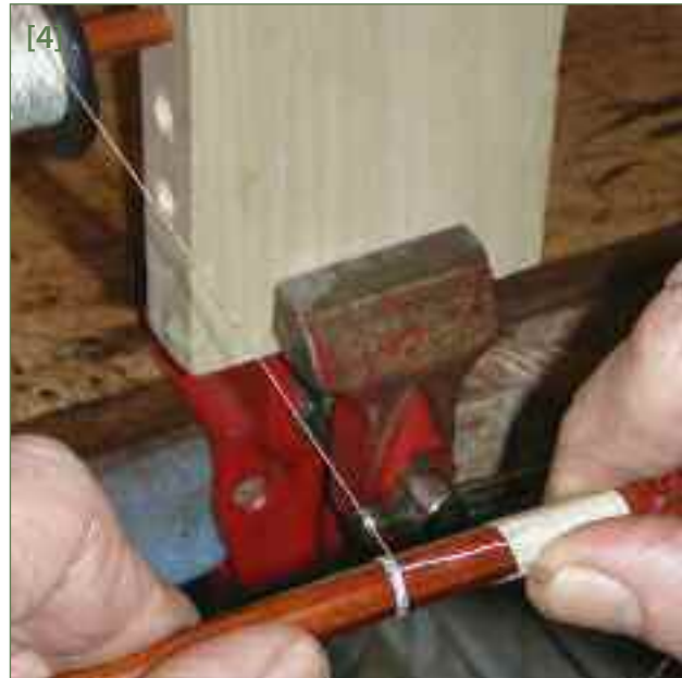
[4] The first three revolutions of spun silver are made
