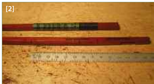
The garniture is planned out on the bare stick with a permanent marker
